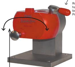
Rotate the handle to lock the tool Positively.
